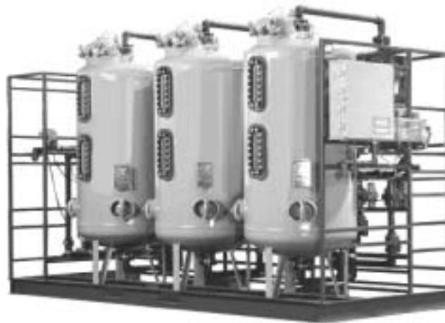
FIGURE 9: Typical Ion Exchange System Composed of Pressure Vessels Filled with Anion Exchange Resin Capable of Treating 75 gpm (Kinetico, Newbury, Ohio)
