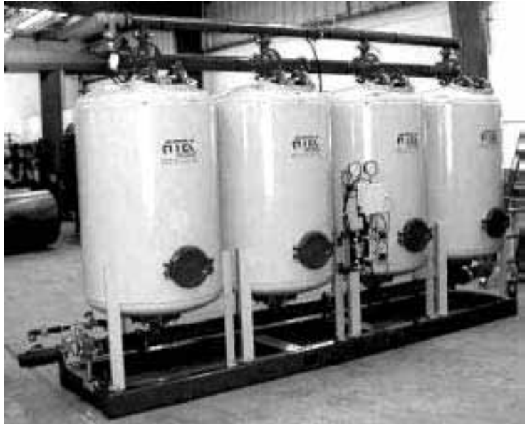
FIGURE 8: Typical Oxidation/Filtration System Composed of Pressure Vessels and Pyrolucite Media for 200 gpm (ATEC Technologies, Hollister, CA)
